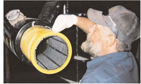
Thordon RiverTough bearings can be bonded or interference fit
